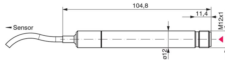
DT3005-x, Abmessungen in mm
