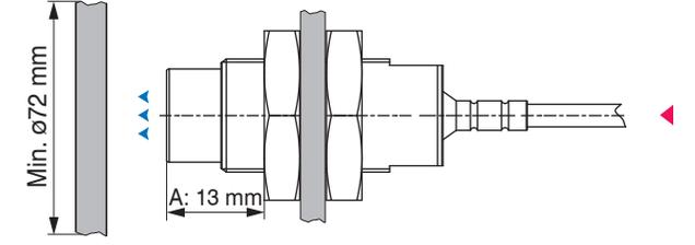
Montage, Abmessungen in mm
